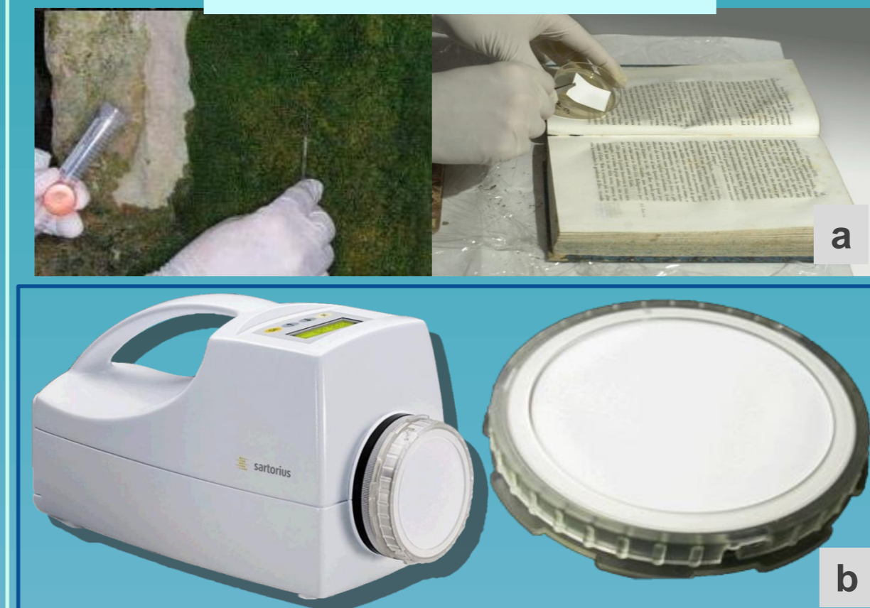
(a) Surfaces sampling by sterile swab and Nylon membrane (b) Air Port MD8 Sartorius equipped with water soluble gelatine filters utilized for aerosol sampling
