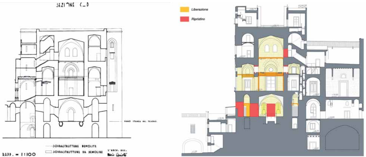
Fig.15 - Vertical section of the the tower (M. Guiotto 1933); Fig.16 - Vertical section: restoration highlighted
