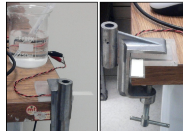
Fig. 6. Pipette, cantilever and vise.
