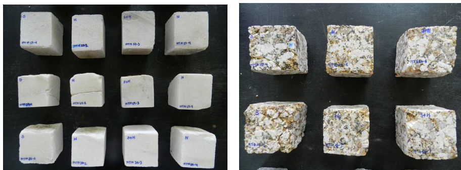
Figure 2 and 3. White marble specimens (4x4cm) mainly used in cornices and capitals. Granite specimens (5x5cm) are found in the basements of the Front stage.
