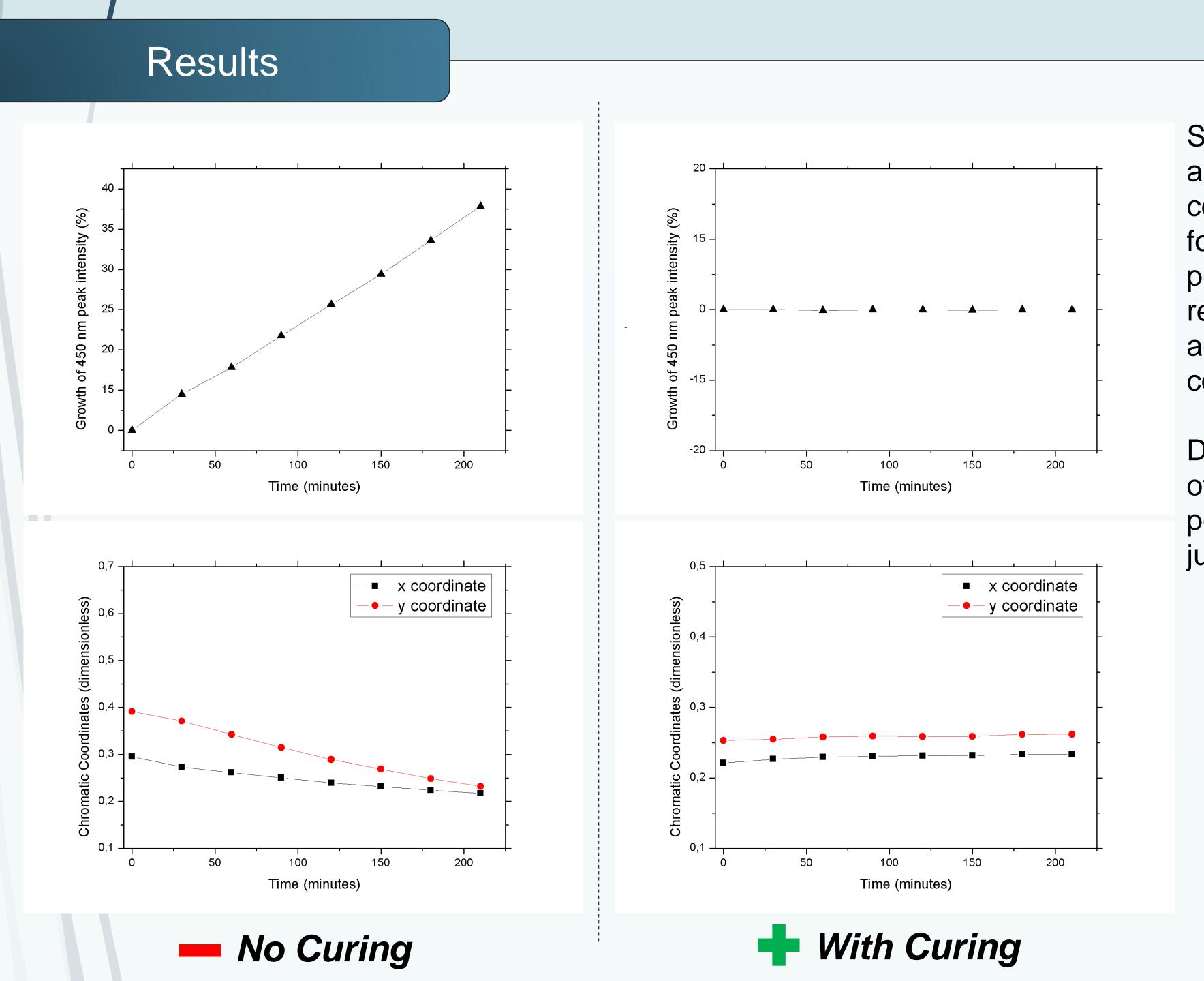
Several tests show that there is a clear difference between a non-cured and a cured mixture. In both cases the spincoated layer of PMMA and Lumogen ® has been irradiated for 210 minutes with a blue LED: during the experiment the percentage growth of the blue emission peak has been recorded, together with the chromatic coordinates according to CIE standards. A white LED with a UV-cured coating does not suffer any spectral variation or color shift.
