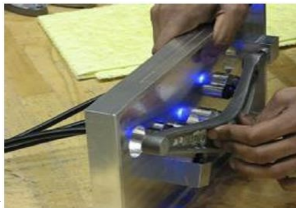
Fig.2-1 Illustration of the photo-curing process used to bond the bracket casting to the PAW
