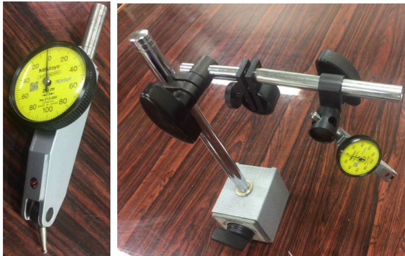
Fig.5-10 Style of dial gauge
