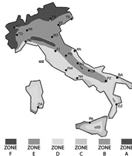
Fig. 3. Classification of the Italian country in Climatic Zones, according to the Italian Presidential Decree n.412/1993 (Source: [6])
