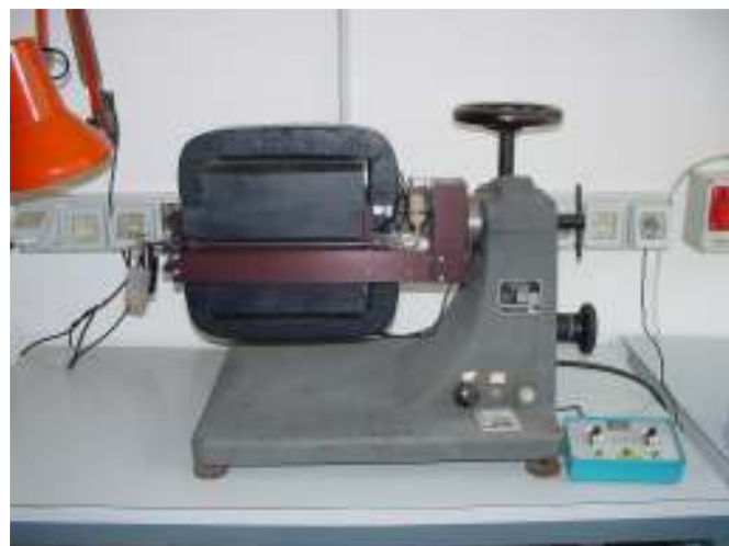
Fig. C.3 – Franz magnetic separator (CFTA)
