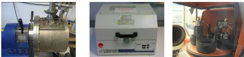
Figure 7.6 The three types of equipment available for the ball milling process; from left to right: attritor mill, shaker mill and planetary mill.
