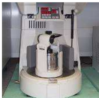
Figure 3.4. Pulverisette series planetary mills: on the left picture, the P6 with one single vial; on the right picture, the P5 able to host up to four vials.
