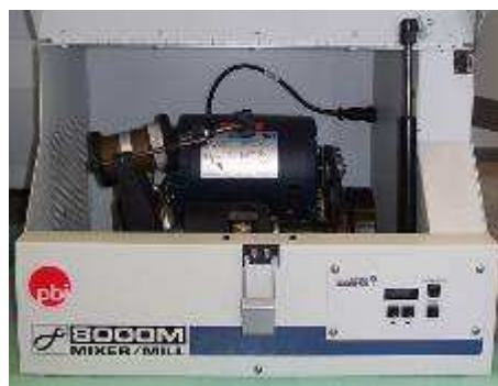
Figure 3.3 Shaker mill SPEX8000N. On the left side the vial's allocation is visible.
