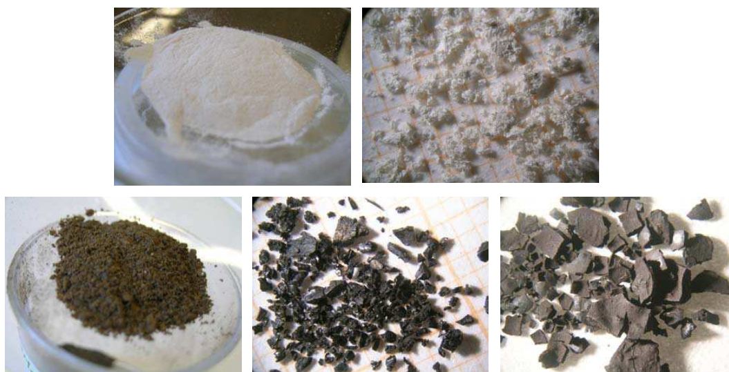
Figure 6.2 Top line: PEEK before (left) and after(right) the chlorosulfonation treatment. Bottom line: the three samples \text{SPMnO}_2\text{-A} (left), \text{SPMnO}_2\text{-B} (centre) \text{SPMnO}_2\text{-C} (right).
