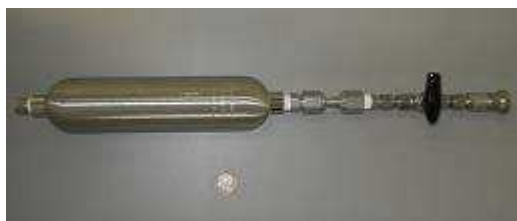
Figure 7.10 The first cylinder of the Nios car's tank: internal volume = 300 ml, amount of material inside = 961 g.
