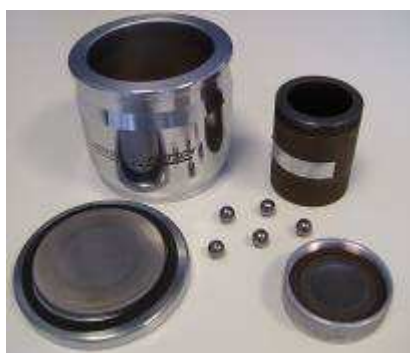
Figure 3.2 Hardened steel milling vials and 10 mm \varnothing stainless steel balls used as milling media.
