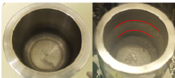
Figure 7.7 The internal view of a planetary mill vial, before (left) and after (right) the milling process: the red lines mark off the region where the hard agglomerated formed on the wall, as well as in the bottom ring.
