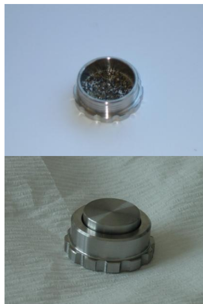
Fig A4 – a) Crusher system at INGV-Palermo b) Steel container of minerals used during crusher procedure.
