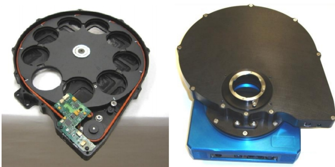
Figure 12: Apogee AFW50-7S filter Wheel mounted on a Apogee UV camera.
