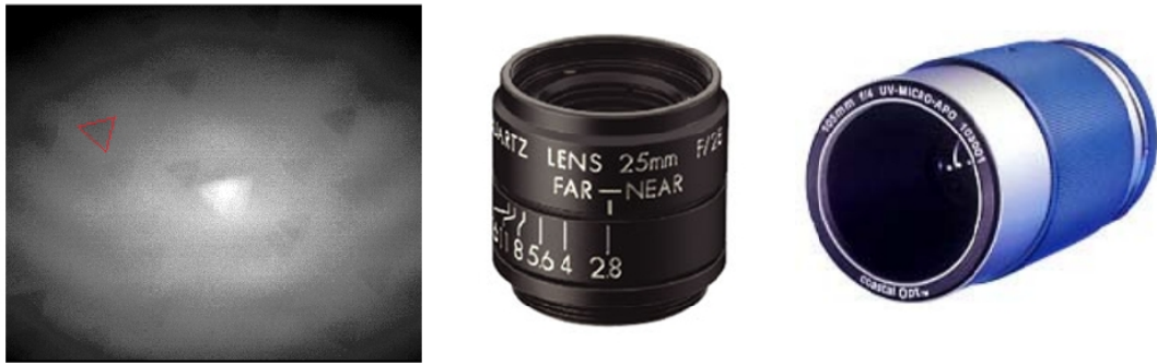
Figure 10: Flare effect on a triangular shaped iris lens and a 25 mm and 105 mm focal length lenses.
