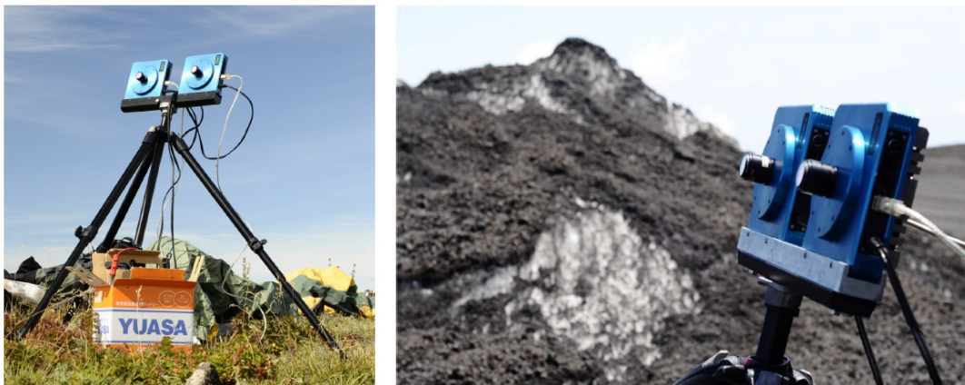
Figure 23: The complete UV camera system adopted in this work.
