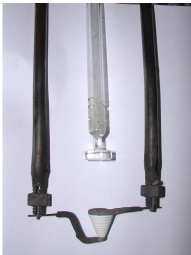
Figure 2.1: The sampleholder in the SMAD apparatus is constituted of a cone rolled tungsten wire, that is linked to two electrodes, covered by an aluminium oxide.
