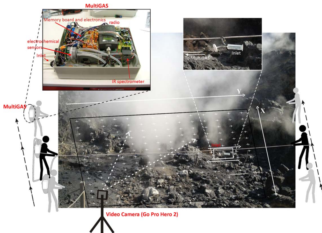
Figure 2. Sketch illustrating the measurement setup. A MultiGAS detector (see inset), held in an operator's backpack, was used to measure (at 0.5 Hz) the composition of the near-vent fumarolic atmospheric plumes. During operations, the inlet of the MultiGAS detector was kept (for \sim 30 – 45 s) at each node of an (x, y) horizontal grid, roughly perpendicular to the vertically ascending gas jet. The grid nodes, separated by 0.5–1 m, were scanned in a step-by-step manner (typically within 1 h) by manually scrolling the inlet up and down a rope tied to the operators (the operators moved stepwise along the x direction of the grid in order to cover the entire grid). A video camera (GoPro Hero 2) pointing toward the vent acquired image sequences of the atmospheric plume at 25–100 frames/s, which were later processed to calculate the time-averaged plume transport speed for each vent (see Table 1).
