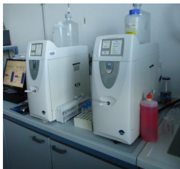
Fig. 37 – Dionex ICS 1100 (image picked in INGV of Palermo).
