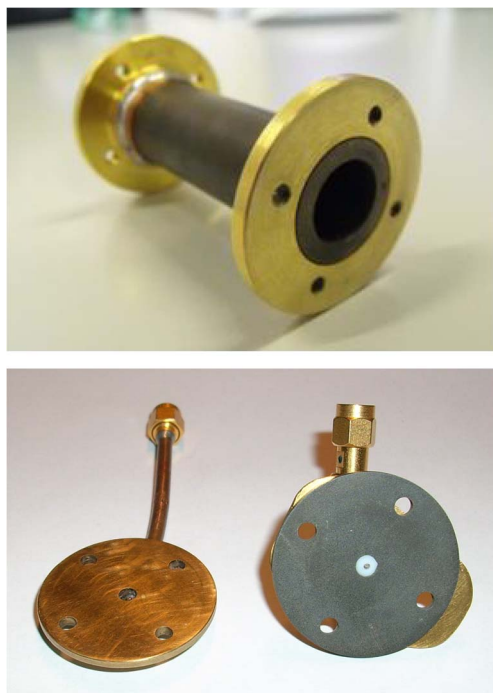
Fig. 2. (Top) A perspective view of the MgB 2 cylinder, which is a part of the homogeneous coaxial cavity; in the image, one can see the two brass rings, successfully soldered by using tin as soldering paste on a thin layer of copper electrodeposited on the outer surface of the MgB 2 cylinder; (bottom left) one of the brass adapters; (bottom right) one of the adapters made using a MgB 2 disk.
