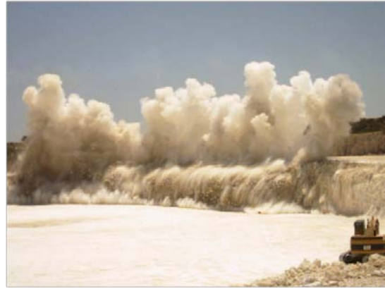
Fig. 5. Extraction through the use of explosives.
