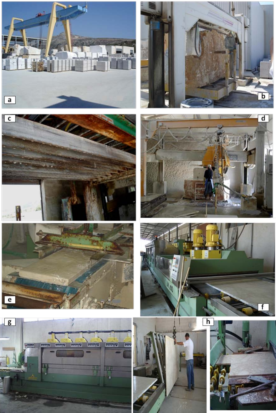
Fig. 10. Description of the phases indicated in Fig. 9. a) Storage of blocks incoming at sawmill, b) single-blade frame, c) multi-blade frame, d) cutting machine, e) splitting machine, f) polishing slabs machine, g) polishing tiles machine, h) polished slab and tile.
