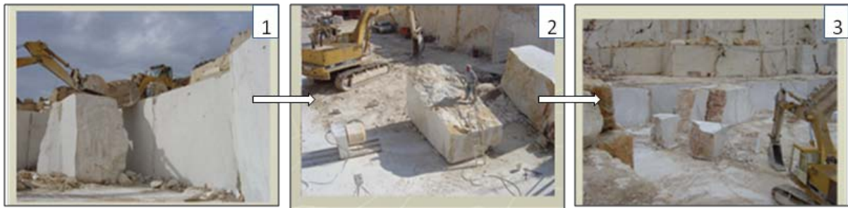
Fig. 6. Description of the phases cited in Fig. 4: tipping and sectioning of the slice.
