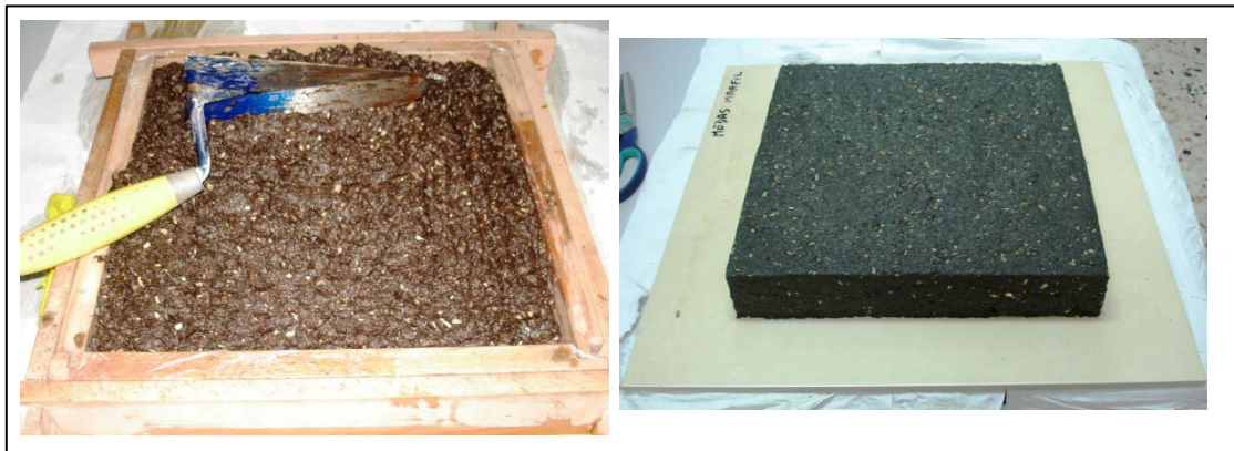
Fig. 2. Positioning of bast-water mixture in the mould (left) and drying of the sample (right).
