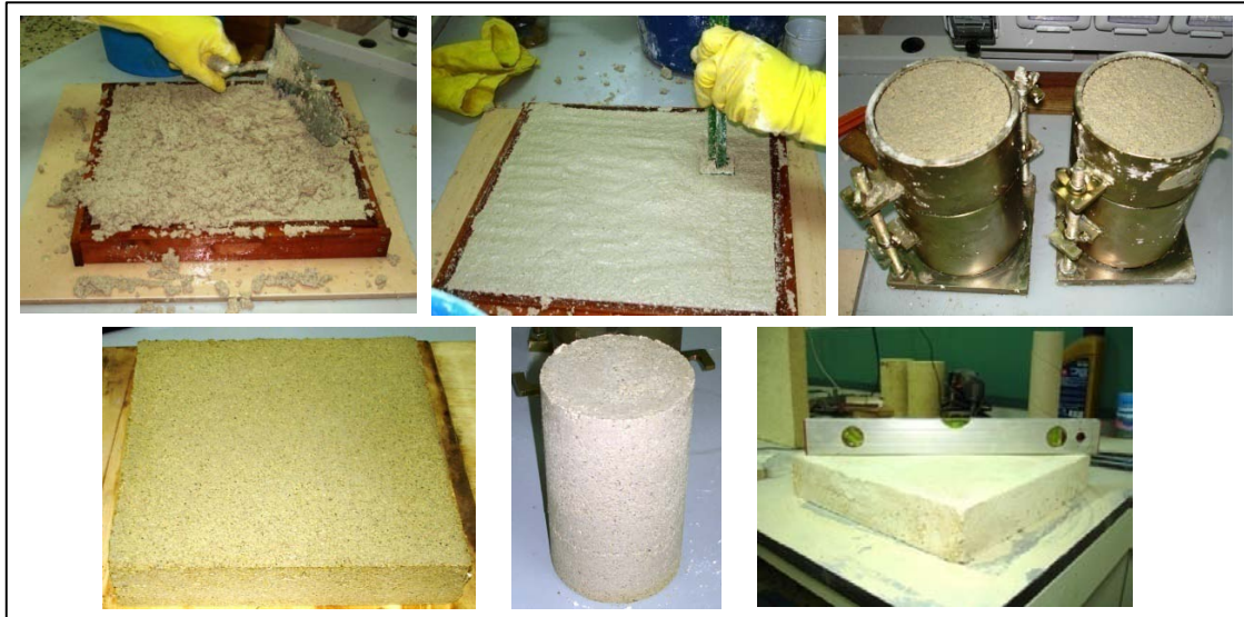
Fig. 4. Cast of hemp-lime mixture in the moulds (upper row) and samples after the drying and smoothing process (lower row).
