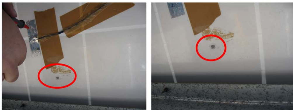
Figure 8. Little holes in the PET film of the PV panel to measure the temperature.
