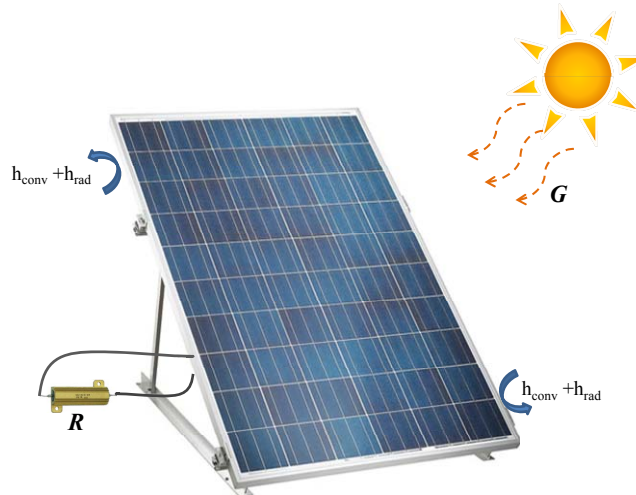
Figure 2. Sketch of energy exchanges of PV panel with surrounding environment.
