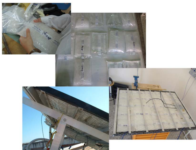
Figure 7. The encapsulated PCM and its installation
