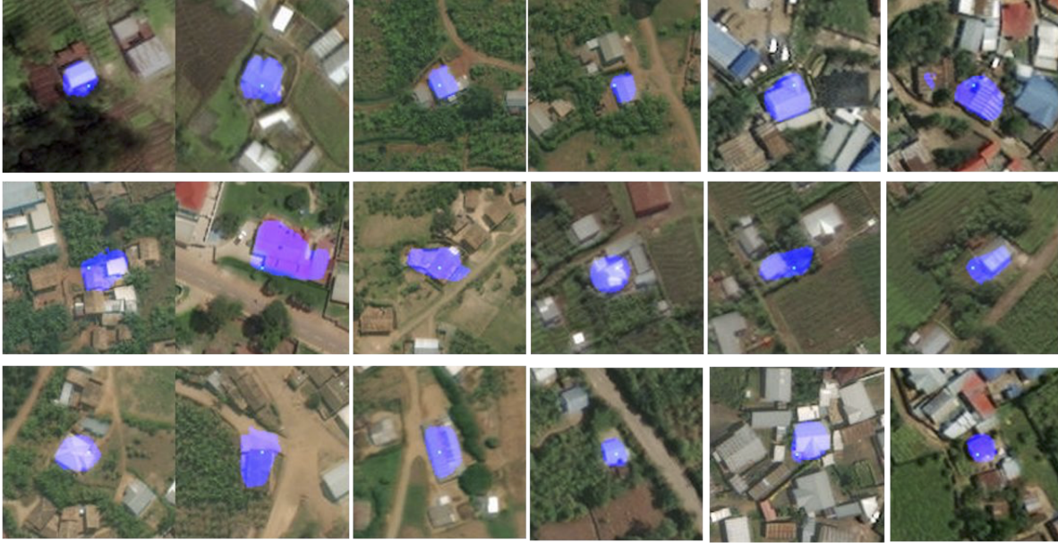
Figure 4.10: Sample building footprints extracted with the Point Segmentation method. Dots show the buildings of interest that are input into the model, while blue outlines shows model outputs as building roof footprint.
