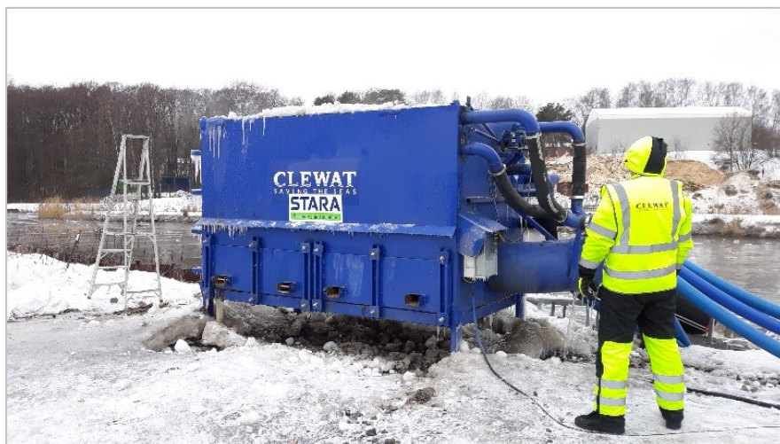
Figure 12. Clewat tested a pilot-scale snow treatment unit in Helsinki in winter 2021. Photo: M. Vahvaselkä.
