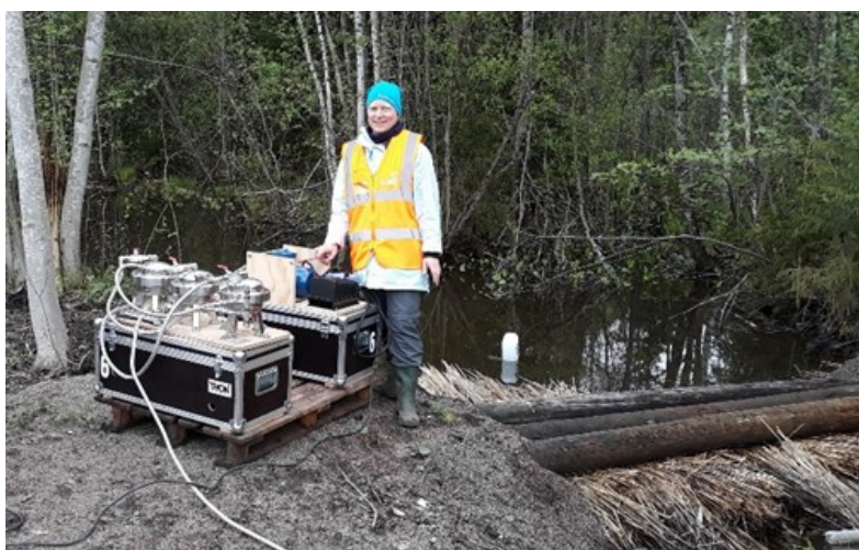
Figure 6. The UFO sampling device from Aalborg University was used for collecting microplastic samples from the ditch water before and after the common reed filter pilot. Photo: M. Vahvaselkä.
