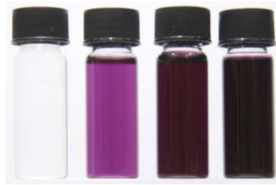
Fig. 2 – Pure tetralin (left) and tetralin containing 0.10356, 0.29953 and 0.65529 mass fraction of fullerene C60 in tetralin (from the left to right).
