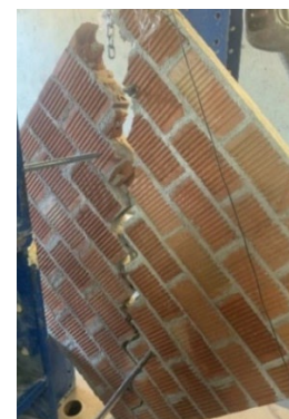
Fig. 8 - Diagonal compression test results, (a) stress-strain plot, (b) failure mode
