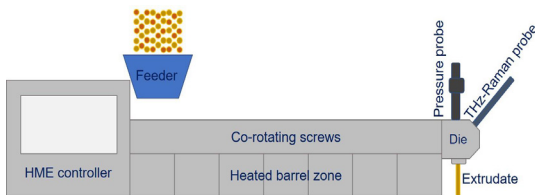
Figure 1 Schematic of extruder coupled with THz-Raman probe*
