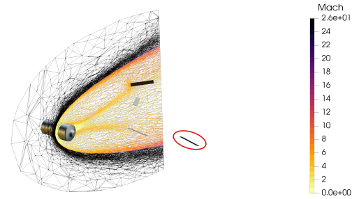
Fig. 10: Fidelity separation at t = 172.8s . Low-fidelity model is used for the circled solar panel
