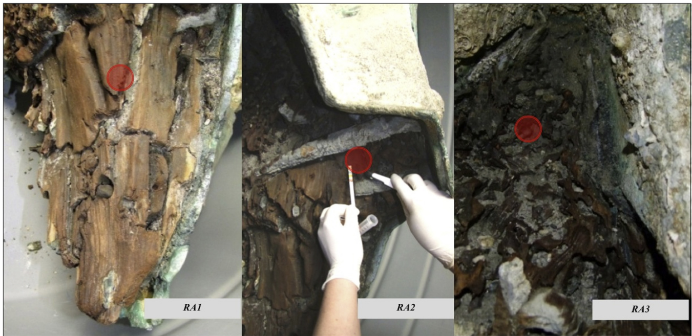
Fig. 1. Wood fragments sampling from different areas (pointed in red) of the wood rostrum structure.
