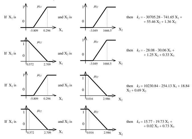
Each rule gives back a value for the output  $ki = f(X_1, X_2, X_3)$ , to which is associated a degree of truth given by  $ki^* = min[\mu 1j(X1), \mu 2k(X2)]$ .  $\mu 1j$  and  $\mu 2k$  are the membership functions characterising the fuzzy subsets defined on X1 and X2. In order to estimate the fuzzy algorithm's output, it is necessary to apply a defuzzyfication method as for example the centroid one:
