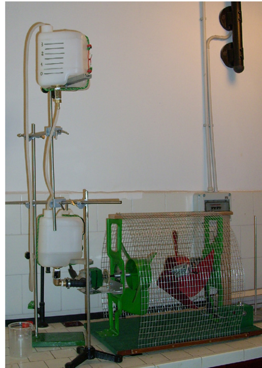
Figure 3. A picture of the experimental apparatus consisting of two fans, a small hydraulic pump and two water tanks.
