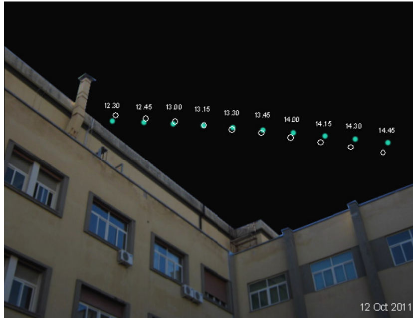
Fig. 10. Comparison between calculated and photographed sun positions on 12 October 2011.
