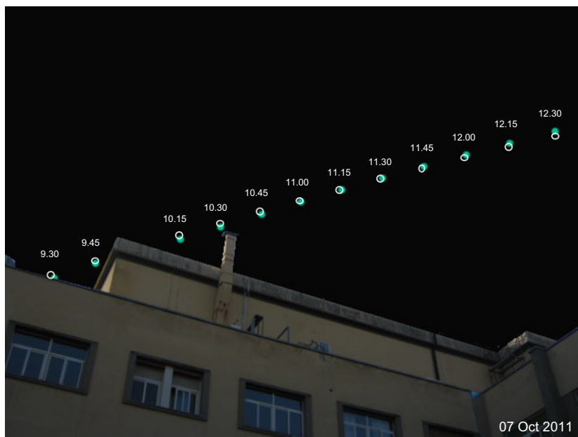
Fig. 9. Comparison between calculated and photographed sun positions on 7 October 2011.
