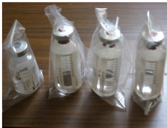
Figure 2. Photograph of calibration bottles containing ^{152-154}\text{Eu} aqueous solution
