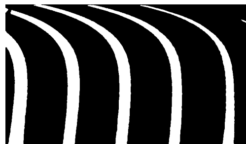
Fig. 18 Binarized isochromatic fringes
