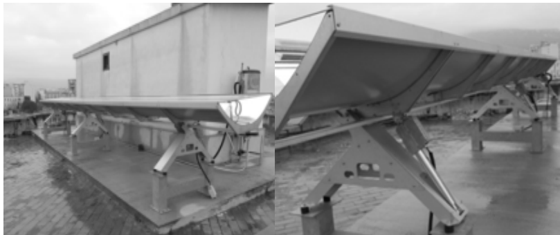
Fig.1: CPVT equipment on the roof of the Energy Department (University of Palermo)
