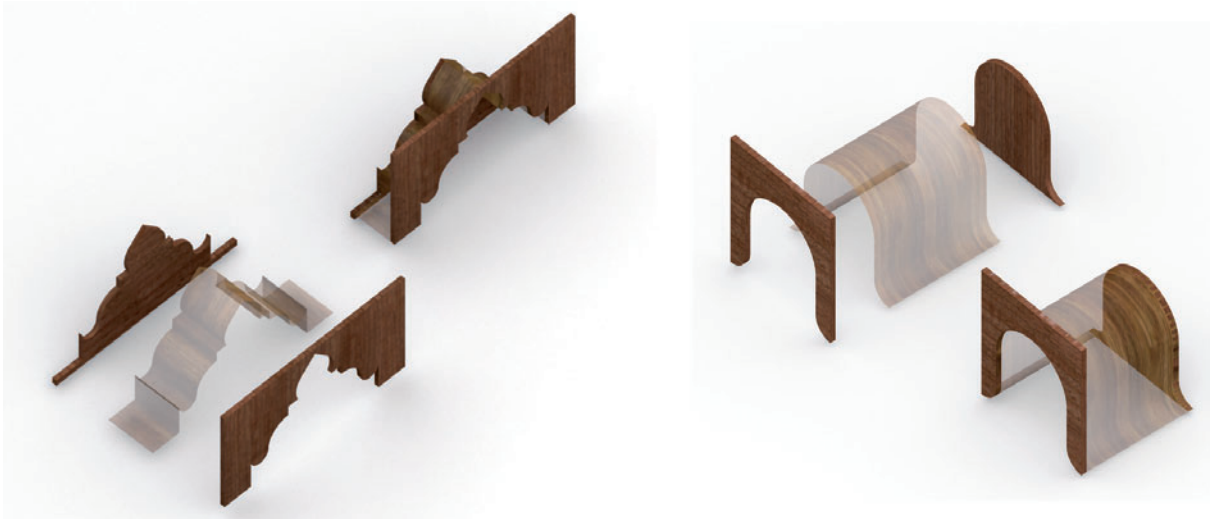
Fig. 52. Fifth tier: constructive layout of polygonal arches (left) and “bonnet” vaults (right). (Images: Fabrizio Agnello and Maria Antonietta Badalamenti)
