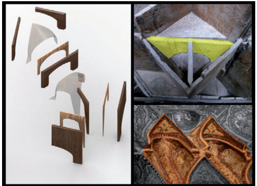
Fig. 37. Third tier: constructive elements of the vaults covering the two right-angled isosceles triangles. The shared hypotenuse is highlighted in yellow. (Image: Fabrizio Agnello and Maria Antonietta Badalamenti; photos of the intrados: Maria Antonietta Badalamenti and Domenico Carbone; photo of the extrados: courtesy of Arch. Mario Li Castri)
