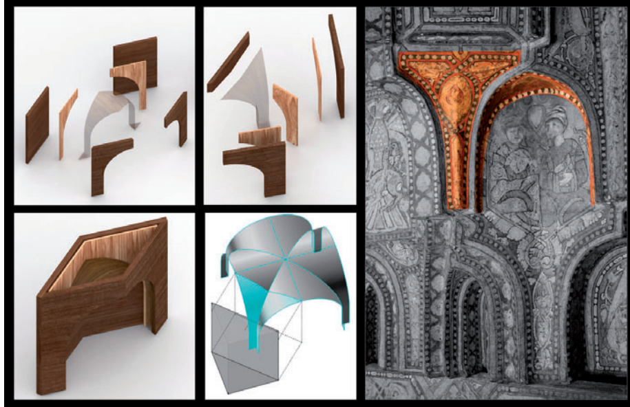
Fig. 31. Second tier. Left) Barrel vaults on rhombs. Middle) Pendentive. Right) Photo with these elements highlighted. (Images: Fabrizio Agnello and Maria Antonietta Badalamenti; photo: Maria Antonietta Badalamenti and Domenico Carbone)
