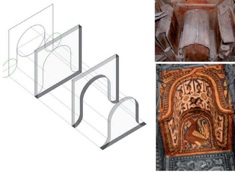
Fig. 40. Third tier: demonstration of hypothesis concerning the construction of the back and front panels in the “bonnet” niche. (Image: Fabrizio Agnello and Maria Antonietta Badalamenti; photos of the intrados: Maria Antonietta Badalamenti and Domenico Carbone; photo of the extrados: courtesy of Arch. Mario Li Castri)
