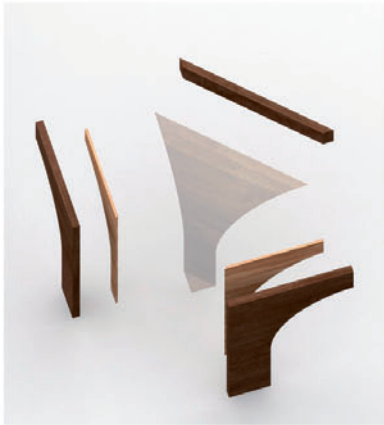
Fig. 27. First tier: the pendentive. (Image: Fabrizio Agnello and Maria Antonietta Badalamenti; photo: Maria Antonietta Badalamenti and Domenico Carbone)
