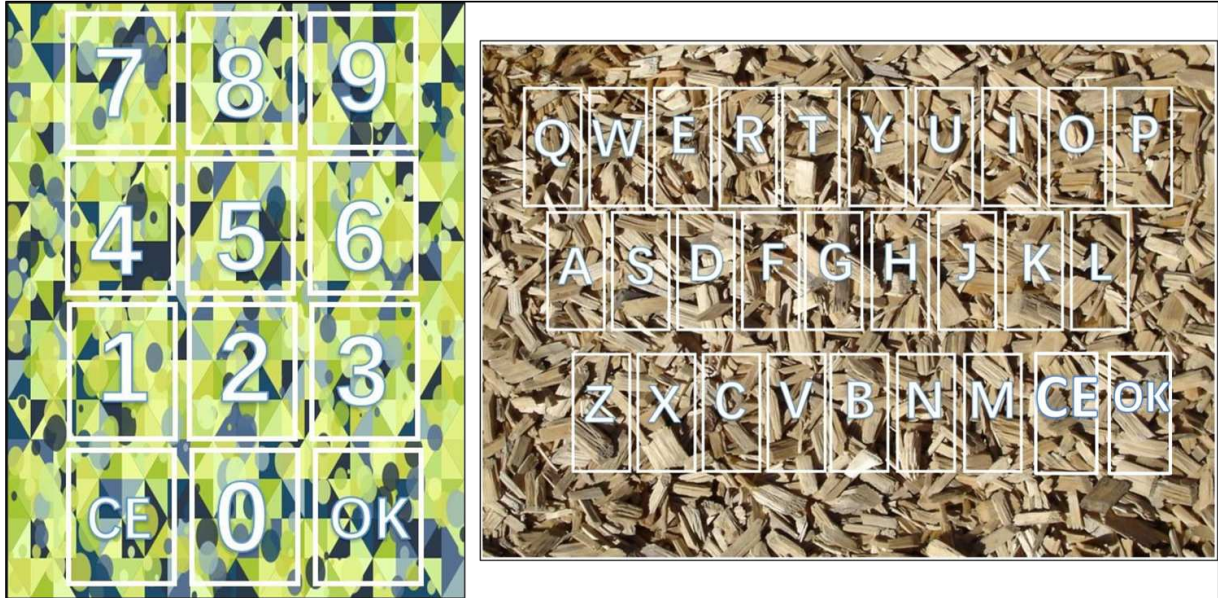
Figure 4.3 Two input markers. They can accept the corresponding input parameters through the user clicking on the marker. The content of each block represents the input information when the user clicks on the block. The CE button is used to delete the last number or character, and the OK button is used as a confirmation button.
