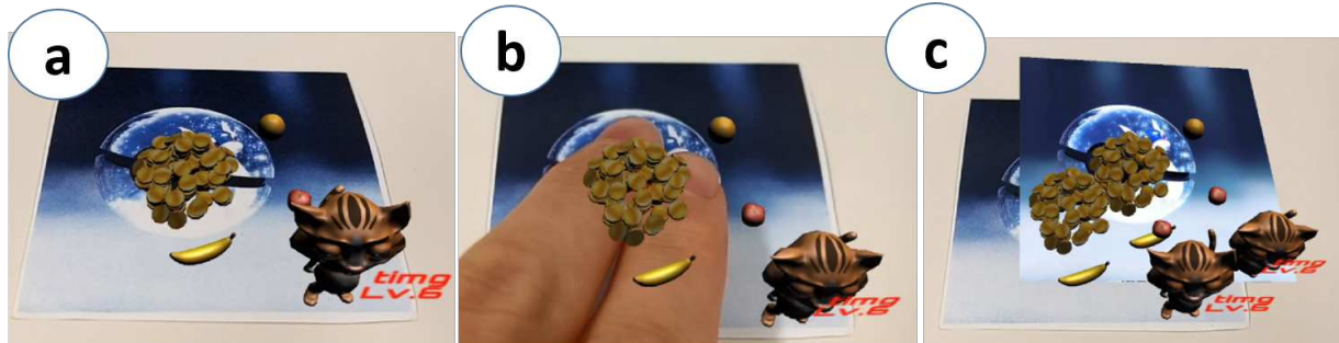
Figure 4.26 A virtual point card generated after touching the physical point card. Pet-based feedback is superimposed on the real point card (see Figure a). The user touches the real point card by hand directly and the card blink (see Figure b). A virtual point card with pet-based feedback is generated after touch (see Figure c).
