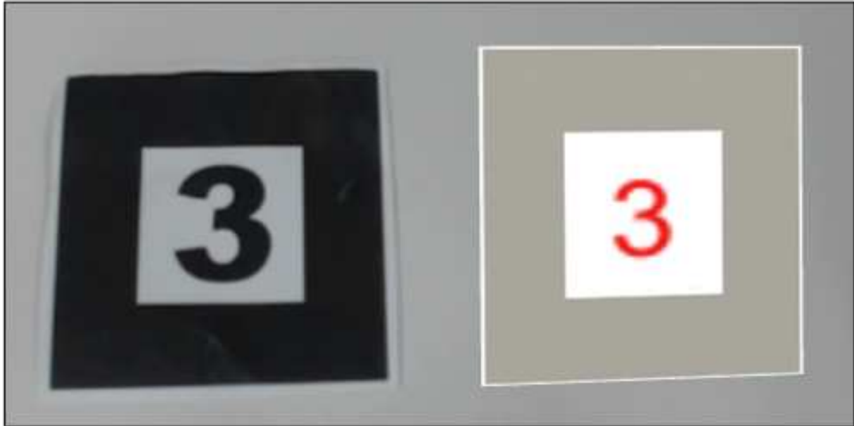
Figure 4.2 Physical and virtual markers. In the AR scene, there is a physical number 3 marker ( left ) and a virtual number 3 marker ( right ). The border of the virtual marker is adjusted to gray.
