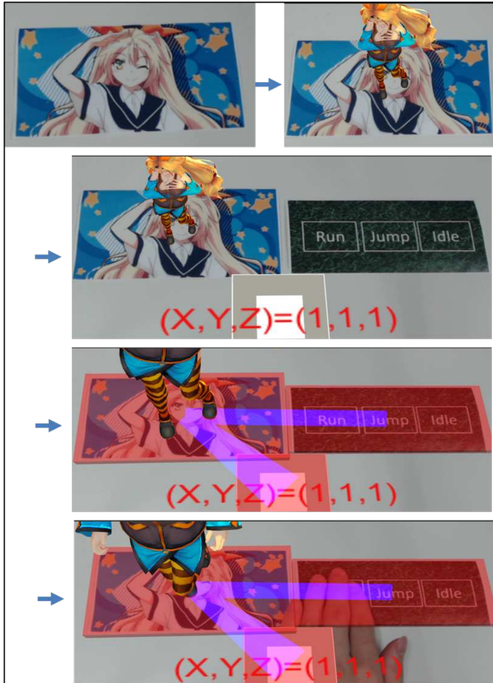
Figure 4.10 Using markers to control the size and movement of the avatar. The first image shows the avatar marker and the second image shows the avatar being superimposed on the avatar marker. The third picture shows the state of the markers before they are connected. After connecting the 3D vector marker and the avatar marker, the size of the avatar will be set to (1, 1, 1), as shown in the fourth picture. In the fifth picture, the user commands the avatar to run by clicking the control marker.
