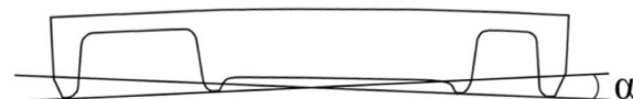
10-3 Measurement points when angle \alpha < 0 , that is, when the two lines intersect on the crown side.
