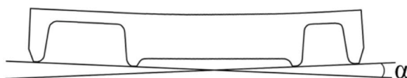
10-2 Measurement points when angle \alpha > 0 , that is, when the two lines intersect on the root side.
