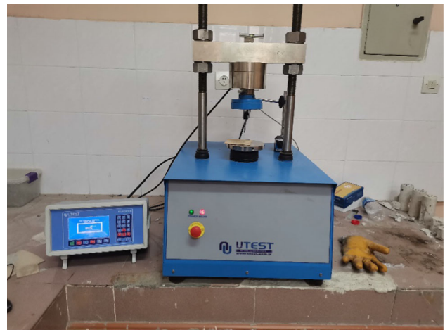
Fig. 6 Unconfined compression test machine
