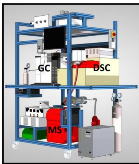
Figure 2.3. Calvet-type in-situ calorimeter with plug-flow geometry Sensys Evo (Setaram) (adopted from[320])
