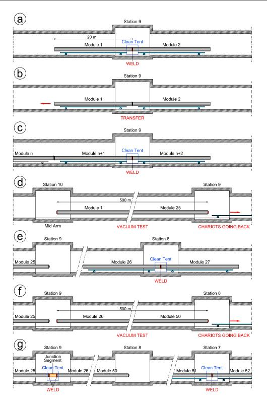
Figure 6.23: The assembly sequence of one vacuum pipe.
