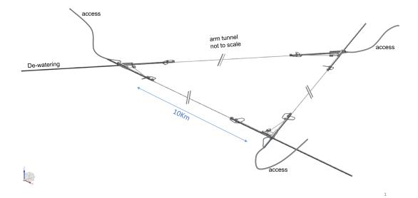
Figure 7.8: 3D impression of the overall tunnel and cavern arrangement for ET. The long tunnels are not shown to scale.
