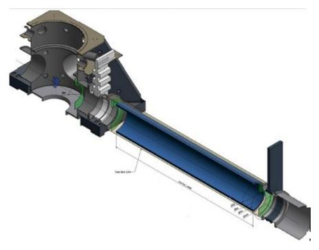
Figure 6.24: A liquid nitrogen cryotrap.
