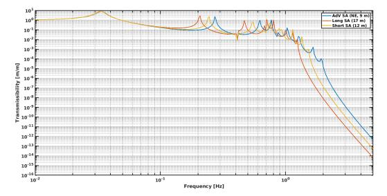
Figure 6.12: Simulation of the SA open-loop horizontal transfer function (Mirror Motion/Ground Motion), along the beam axis, in different configurations. Advanced Virgo SA (blue curve) is compared with two longer versions: 17 m (red curve) and 12 m (orange curve).
