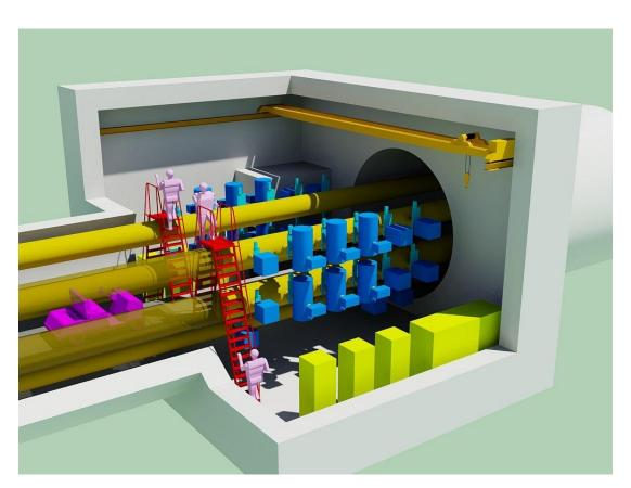
Figure 6.22: 3D view of a pumping station: the blue objects represent the pumps and sensors, the yellow ones the cabinets for pumps control and baking power supply (1 cabinet for all). A separate small room is reserved for the high voltage electrical transformer.
