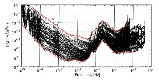
Figure 7.2: Overlay of network station spectra used in Peterson's background noise study [15] together with straight-line segments fitted to the high-noise and low-noise envelopes of the overlay.
