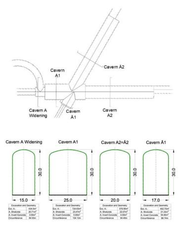
Figure 7.15: Cross section of Cavern A, image source Implenia.
