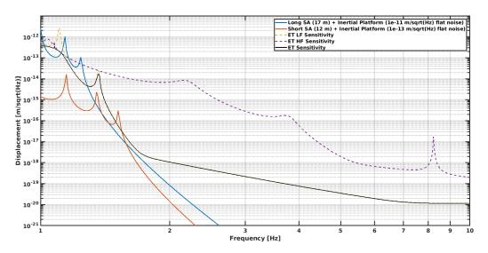
Figure 6.13: The simulated mirror displacement obtained using a 17 m-SA and 12-m SA installed on ideal sensor limited-inertial platform with different requirements (blue curve and red curve respectively) is compared with ET-LF, ET-HF, and the combined ET sensitivities (orange, magenta, and black curves respectively).
