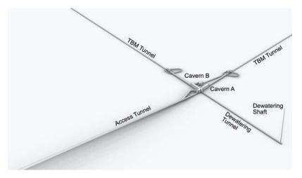
Figure 7.9: Sketch of a layout with inclined tunnels for access to the vertex stations. "TBM Tunnel" indicates the arm tunnels of the triangle, produced with a Tunnel Boring Machine.
