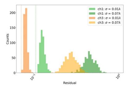
Figure 7.6: Suppression of NN from body waves with 15 single-axis (ch1) and three-axis (ch3) seismometers. Sensor locations of 500 arrays for each histogram are derived from the optimal array by adding random numbers to all optimal coordinates drawn from Gaussian distributions of width  $\sigma$ . Vertical lines mark the residual of the optimal arrays. Plot from [16].
