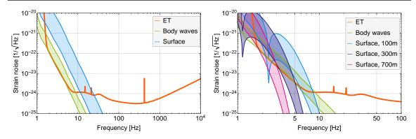
Figure 7.4: Estimates of seismic NN for ET. Left: ET constructed at the surface. Right: ET constructed underground.
