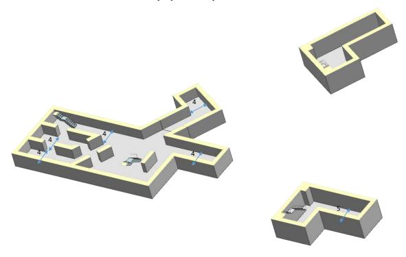
Figure 7.13: Example layout of the basement level of Cavern A with entrance rooms and reinforcement walls giving a solid support for the vacuum tank bases.
