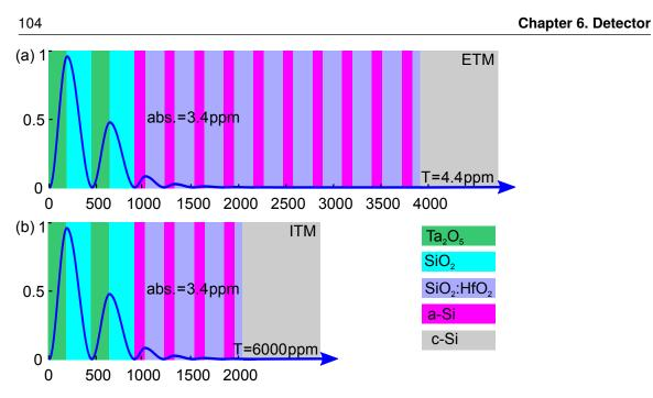
Figure 6.5: A multimaterial coatings design for (a) an ETM and (b) and ITM. This design uses an upper stack of  $SiO_2/Ta_2O_5$  on top of a  $SiO_2$ :HfO<sub>2</sub>/aSi lower stack [12]. The blue lines show the electric field intensity as a function of depth in the coating.
