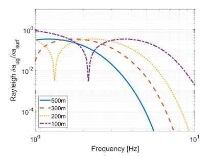
Figure 7.3: Suppression of Rayleigh-wave NN with depth. In this model, it is assumed that wave speed falls from 1.8 km/s at 1 Hz to 500 m/s at 10 Hz. These suppression curves are used in the right plot of Figure 7.4.
