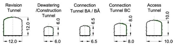
Figure 7.22: Sizes of connection tunnels. Image source Implenia.
