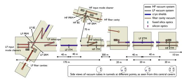
Figure 6.4: Sketch of the optical layout in one corner of the triangle of ET. One can notice in particular the geometrical design of the recycling cavities featuring folded telescopes between the beam splitter and input mirrors. The acronyms used are detailed in the text.
