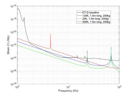
Figure 6.14: Strain sensitivity due to suspension thermal noise for the room temperature and cryogenic suspensions; red: room temperature silica, blue 120 K silicon, green 20 K silicon, black ET-D baseline
