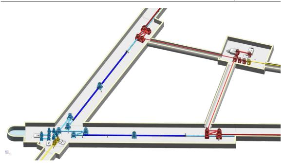
Figure 6.17: One corner of the ET vacuum system: LF dectector (blue); HF detector (red); filter cavities (yellow).
