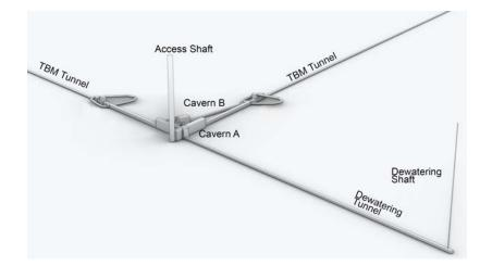
Figure 7.10: Sketch of a layout with vertical shafts for access to the vertex stations. Image source Implenia.
