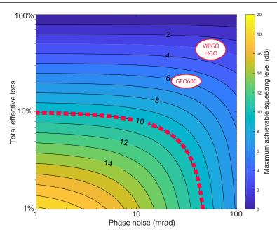
Figure 6.6: Maximum effective squeezing level as function of phase noise and optical loss. In order to reach the goal of 10 dB detected squeezing, the optical loss needs to be smaller than 10 % while the phase noise must not exceed 10 mrad.
