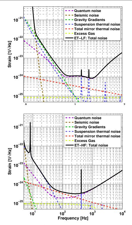
Figure 1.13: Noise budget for the low-frequency (top) and high-frequency (bottom) interferometer for the parameters stated in table 6.1. Shown in black is the amplitude spectral density of a gravitational wave required to produce a signal with the same strength as the total noise of the interferometers. The total noise is decomposed into the individual noise sources, which being statistically independent add up quadratically.
