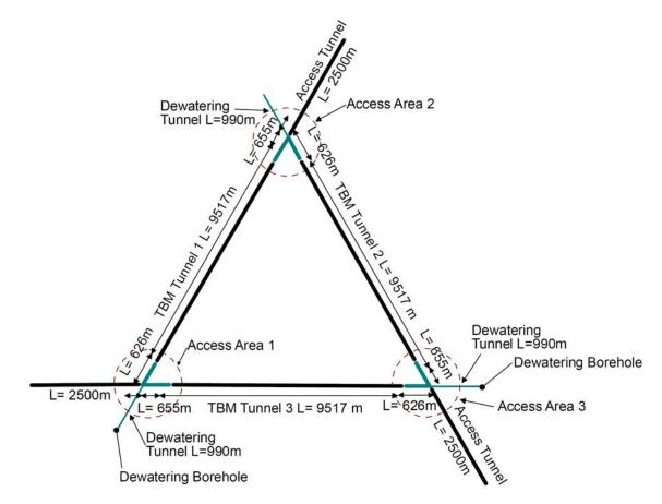
Figure 7.7: Underground infrastructure of ET. Cavern groups (shown in cyan) are connecting by the long tunnels forming the ET triangle. About 1 km long de-watering shafts also contain Filter Cavities. Each corner station is accessible by an access shaft or tunnel. The image shows the lengths of the various sections. Although accurate numeric values are shown here, the detail led length requirements need to be determined in the technical design phase. Image source Implenia.
