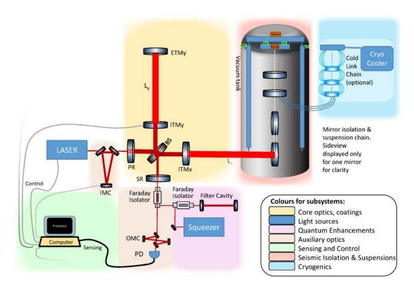
Figure 1.1: Schematic representation of an interferometric gravitational wave detector. Subsystems are indicated by the colored backgrounds. The borders between subsystems are not sharply defined and somewhat arbitrary.
