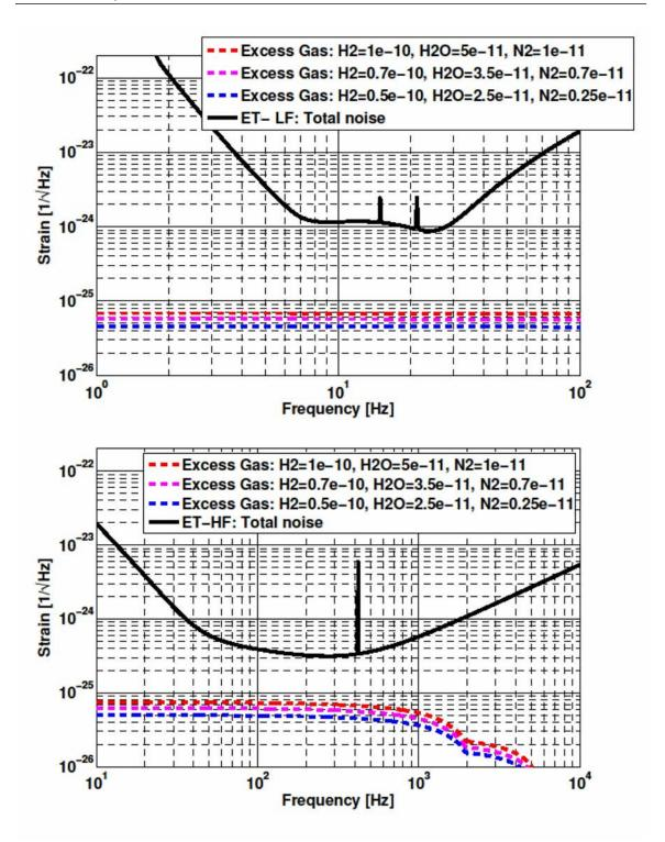
Figure 6.16: Phase noise given by the residual gases compared to the expected sensitivity, computed for the appropriate beam profile for different gas compositions. (Goal gas composition: Hydrogen [ $1 \ 10^{-10}$  mbar], Water [ $5 \cdot 10^{-11}$  mbar], Nitrogen [ $1 \ 10^{-11}$  mbar])
