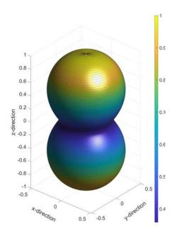
Figure 1.9: The normalised antenna pattern (amplitude sensitivity) of the combined three detectors of the Einstein Telescope for unpolarised waves, i.e. the quadrature sum of "x" and "+" polarised waves.
