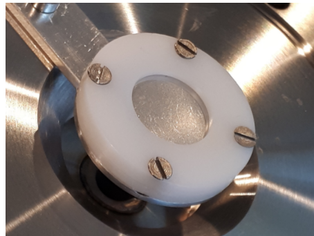
Figure 3.3: Photograph of the implanted stainless steel sample inside the holder used for the spectrometric measurements.
