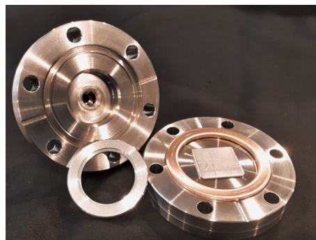
Figure 3.7: Photograph of the vessel used for the radon emanation measurements of the implanted stainless steel samples. The aluminum ring in the front is used to fix the sample in place.
