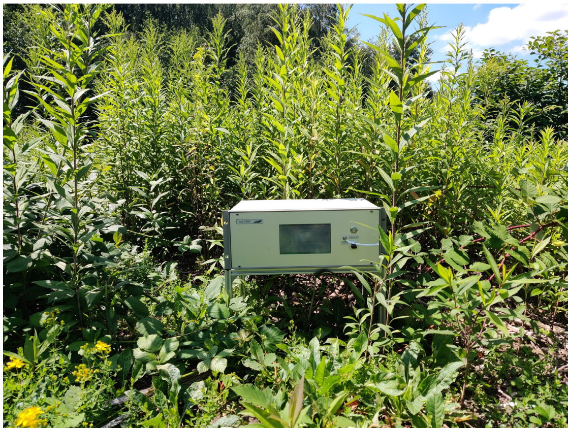
Fig. 10. The mobile GC-IMS can undertake pVOC-measurements directly on site. The current setup is equipped with rechargeable batteries and an internal, close gas circuit for 4 h of autonomous operation independent of a local energy source..
