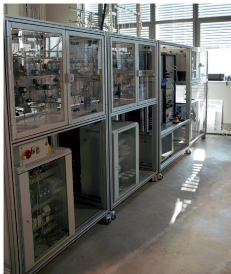
Figure 3. Overview of the structure of the gas generator subdivided into individual plant parts from left to right: the two gas supplies, the liquid dosing station and the analysis section.
