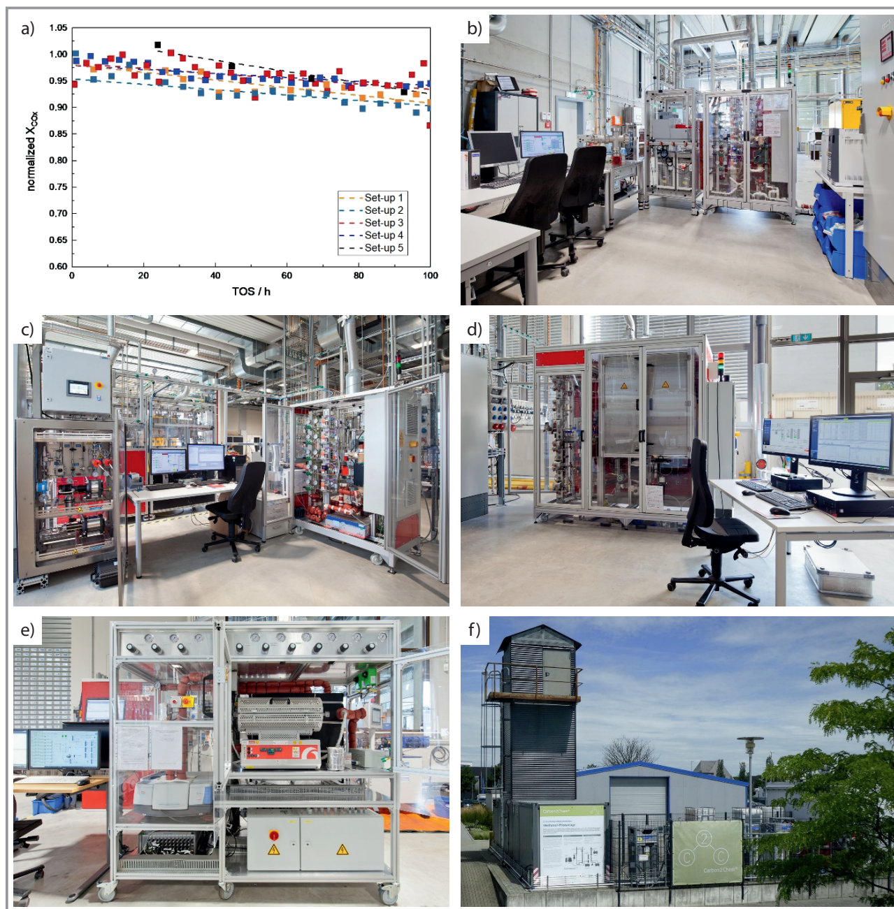
Figure 4. a) Normalized degree of conversion of CO x (X CO x ) of the standardized benchmark test for methanol synthesis over an industrial Cu/ZnO/Al 2 O 3 catalyst in the applied setups at 523 K and 50 bar. b–e) Setups used in the Carbon2Chem ® laboratory of MPI CEC and RUB for methanol synthesis as well as f) Fraunhofer UMSICHT demonstration plant for methanol synthesis at the location in Oberhausen.
