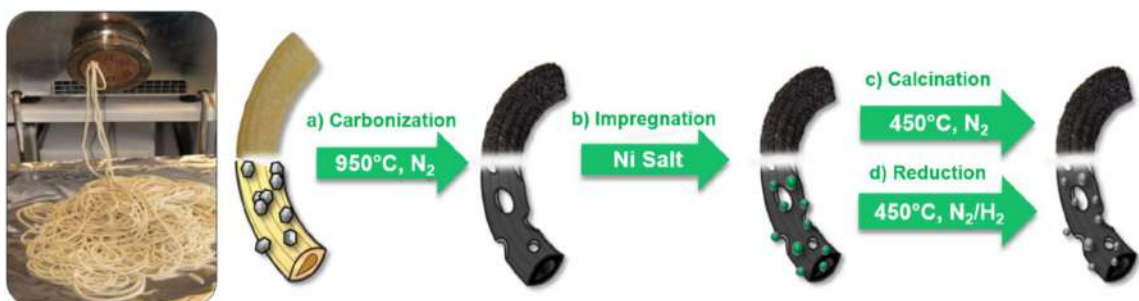
Figure 3.1. Schematic representation of the catalyst synthesis protocol starting from the extrusion, carbonization, calcination, and reduction steps.
