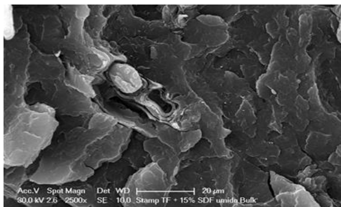
Fig. 6. SEM micrograph of an injection molded SDF sample
