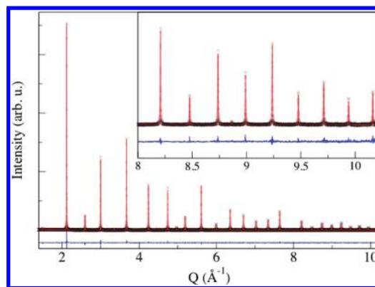
**Figure 2.** XRD data and model for undoped BZ.
