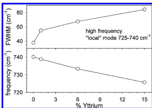
**Figure 16.** Variation of the position and width of the Raman peak at 740 cm<sup>-1</sup> as a function of dopant content.
