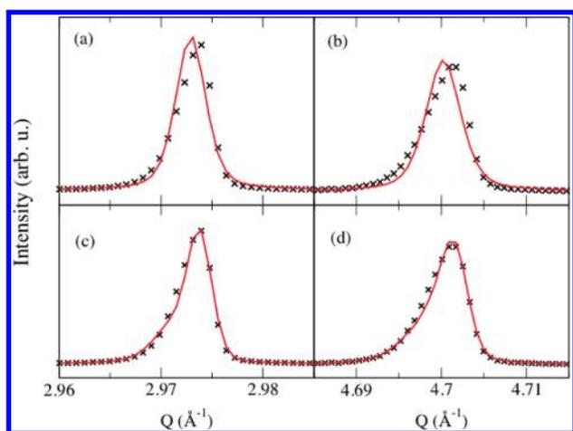
**Figure 1.** Comparison of the XRD best fitting for BZY15HYD, obtained with cubic (panels a and b) or tetragonal (panels c and d) models. The two peaks correspond to the (200) and (310) reflections of the cubic unit cell, respectively.
