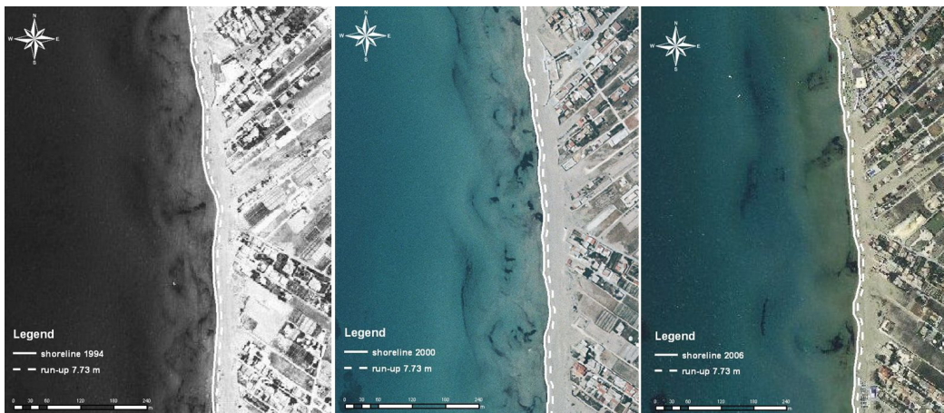
Fig. 4. Shoreline position and maximum run-up during the 1994 (left panel), 13/05/1999 (central panel) and 27/08/2005 (right panel) acquisitions.
