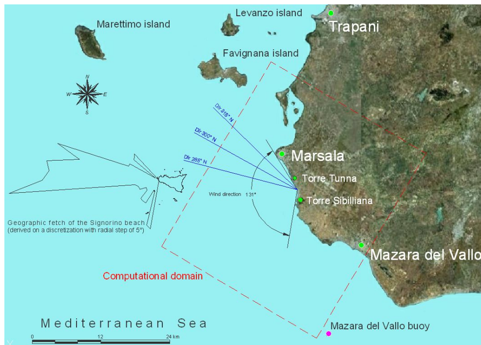
Fig. 1. Computational domain (dashed line) of the study area, with wind and critical wave directions.
