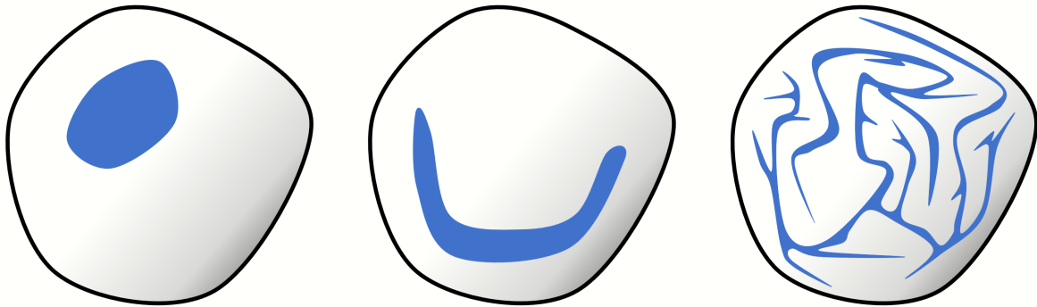
Figure 2.1: Schematic drawing of the evolution of a set of phase space points (blue) evolving on an energy shell of H_0 (shaded shape). As time moves forward from left to right, the set shifts and stretches while maintaining a constant phase space volume, as required by Liouville’s theorem. After enough time, the set is fibrillated across the entire energy shell, and is uniformly distributed across the shell at a coarse-grained level.
