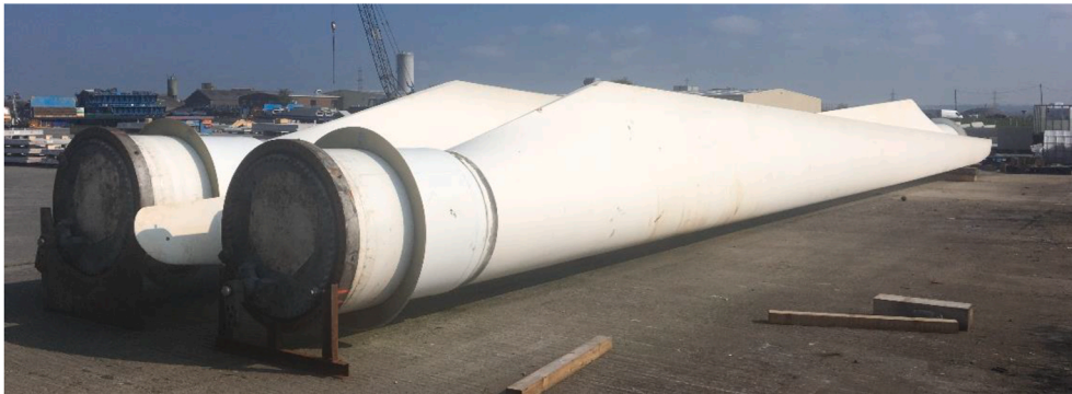
Fig. 4. An example of a blade approximately 21 m in length (photo credit Emma Delaney).
