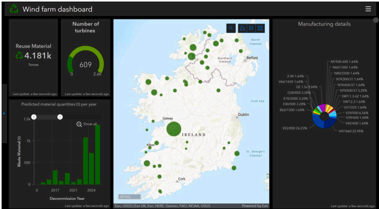
Fig. 3. Dashboard depicting Irish wind farms that are 16 years or older (Delaney et al., 2021).
