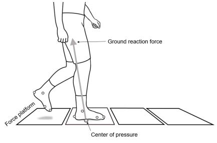
**Figure 1.** Experimental setup (at UAMS) showing four force platforms which were used to assess center of pressure (COP) movement during single-support phase (only one limb is in contact with the ground) of walking.
