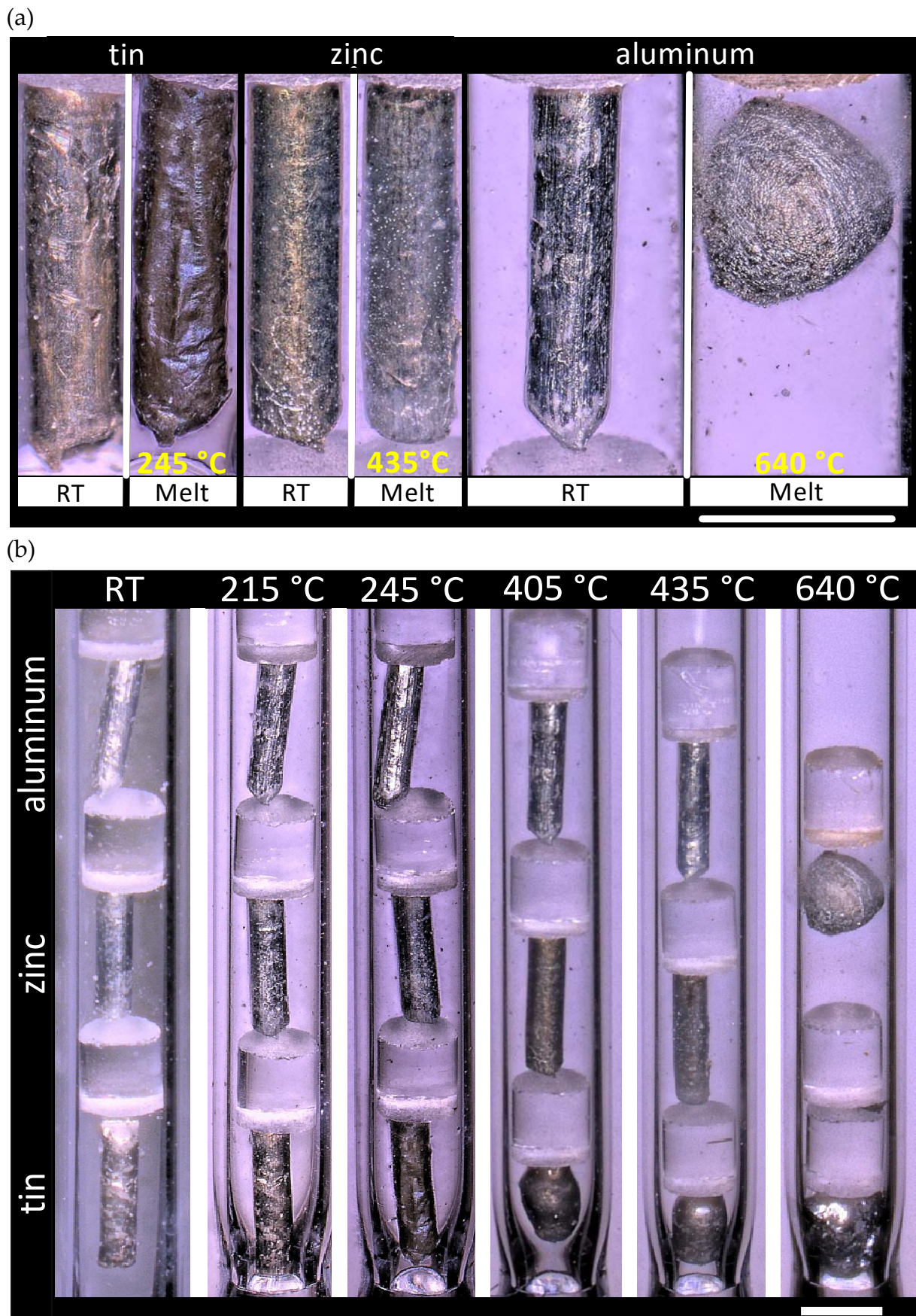
Figure 5. Standard melt wire capsule furnace testing: magnified view of the visual temperature response indicating melting of (a) individual melt wires of Sn, Zn and Al, and (b) of the full capsule. Scale bars represent 1 mm.
