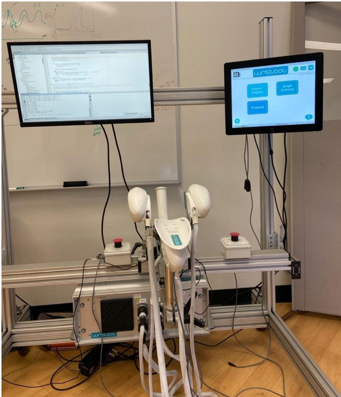
Figure 5. WristBot Set up. System interface screen (right), WristBot device (middle)
