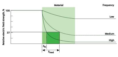
**Figure 2** How EM RF energy is absorbed by biological materials, i.e. how skin depth decreases with higher frequency. Reflection of the incident radiation is assumed negligible at each interface in this diagram. Skin depth at high frequency,  $\delta_{hi}$ , is less than that at medium frequency,  $\delta_{med}$  (14, 16)
