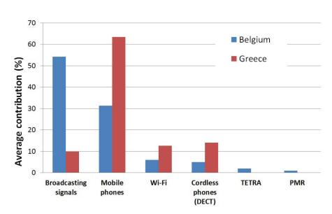
**Figure 1** Average contribution (%) of various RF signals measured as electric field strength (V/m) in Belgian and Greek schools (7)
