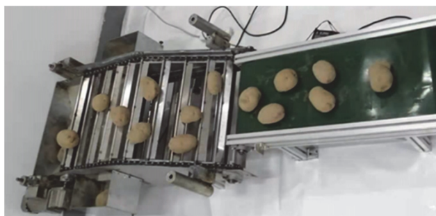
Figure 7 Test bench of rod-type conveyor grading device
