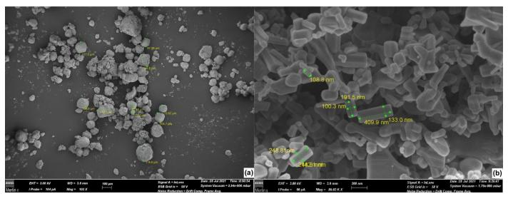
Figure 1. (a) Micrometric clusters of ZnO nanoparticles present in untreated dust and (b) ZnO nanoparticle size after sonication treatment (FESEM microscopy).
